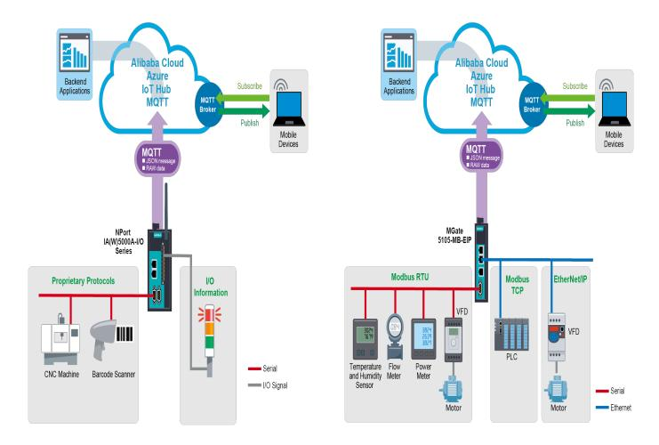
Furthermore, Moxa's device servers and protocol gateways not only offer multiple serial-to-cloud combinations, but are also desgined to simplify
