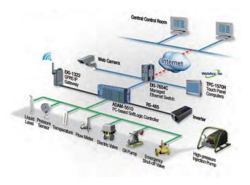
The main function of an intelligent remote supervisory system is to monitorthe operating status of local and remote intelligent equipment. WebAccesssoftware manages and controls the water injection pumps & valves, theparameters of intelligent equipment such as the temperature and pressureof lubricating oil; valve opening angles; the details of valves, alerts and theopen/close functions. WebAccess? powerful network functions are perfectfor on-site and remote monitoring of intelligent equipment.
