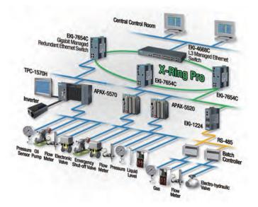
systemuses a unified control module to control all the points of the oil terminal andensure data transmission quality and safety whilst being compatible with othersystems such as ERP.
