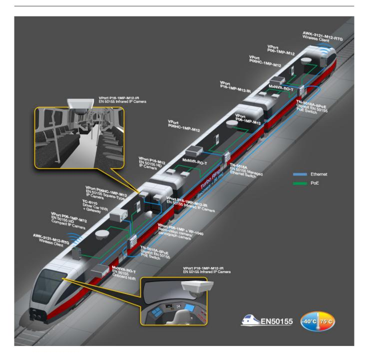
IP-based CCTV systems are becoming an absolute requirement for metro operations. Effective video surveillance protects passenger safety and makes metro operations more efficient, which has led to increased investment in onboard IP CCTV systems. These systems have expanded in scope and reach, and cameras and
